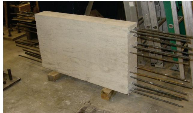
Precast HPFRC coupling beam (note that reinforcement exits the beam horizontally)
