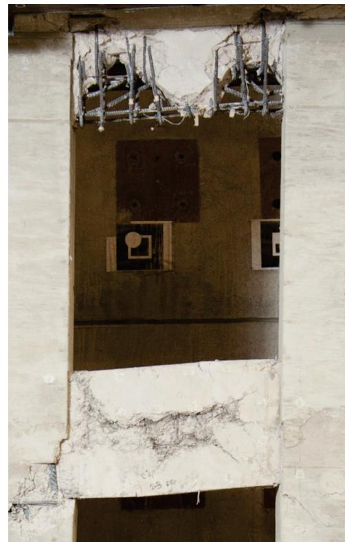
Damage in link beams after being subjected to earthquake-type loading. Top: regular concrete link beam; Bottom: HPFRC link beam
